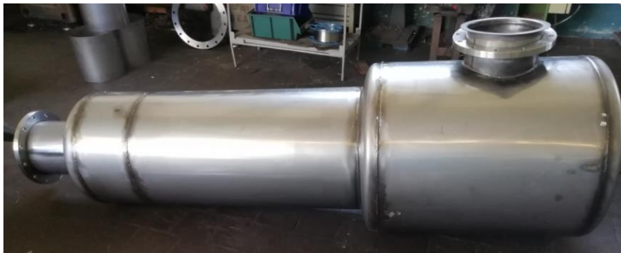
RD silencer made of 304 Stainless steel
